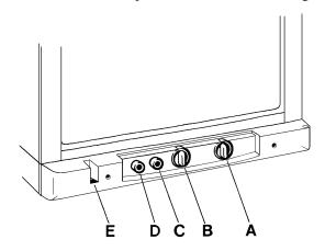
The energy selector (A) can be set at "ELEC" (120 volt AC), "GAS" (LP gas) or "OFF". The refrigerator temperature is controlled by a thermostat (B). Please note that the thermostat has no "off" position.
