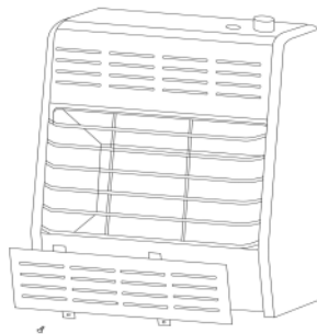
Figure 7 - Removing Lower Front Panel Of Heater
